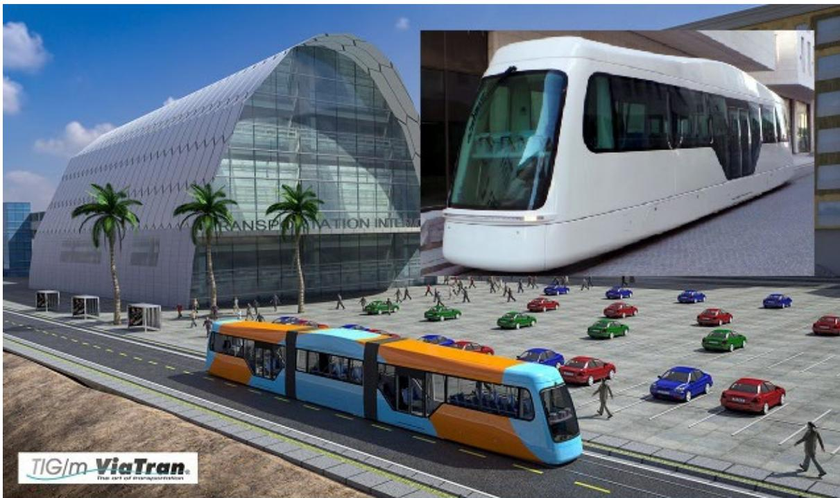
**New light rail transit: there is no longer any need for overhead wire - each vehicle is self-powered by a battery and can operate for 20 hours on a single charge**
